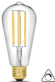
ST64-Clear WATTAGE: 6.0W LUMEN: 660LM CCT: 2700K VOLATGE: 220-240V SIZE: 64X140MM
