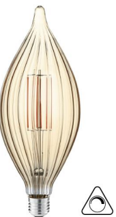
R100-Amber WATTAGE: 4.0W LUMEN: 320LM CCT: 2700K VOLATGE: 220-240V SIZE: 100X255MM
